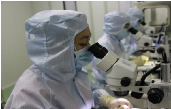
In-process Stent Inspection
