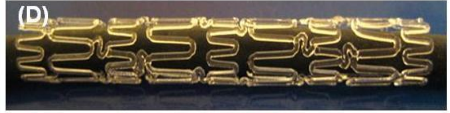
PLLA stents: (A) helical; (B) closed-cell; (C) zig-zag; (D) complex.
